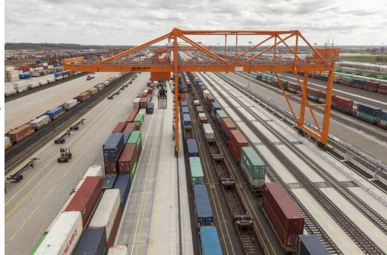
Electric cranes moving containers and trailers between trucks and trains at intermodal yard
